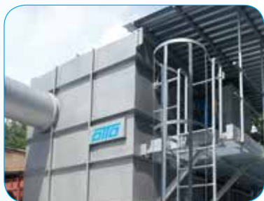
Production of abrasives Air flow rate: 27000 Nm 3 /h Pollutants: phenol, formaldehyde, ethanol
