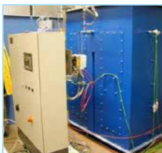
Pilot plant of a regenerative thermal oxidiser (RTO) type Regetar P Flow rate: max. of 300 Nm 3 /h material for heat recovery: material with a honeycomb structure or in bulk
